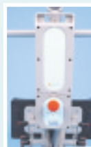
Electrics have clearly visible controls including emergency stop
